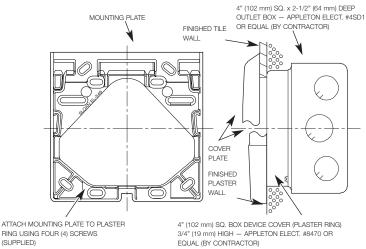
To ensure a perfect rough-in, Sloan recommends the use of the EL-518-A Flushometer Electrical Box Positioning and Support Kit. Specify and order the EL-518-A Kit separately. Consult factory for installation details.
