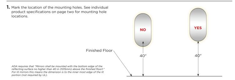
Install included #14 round slotted wood mounting screws into pre-marked holes. Note, all mirrors must be installed in contractor supplied blocking. Slide the mirror assembly onto the screws.
